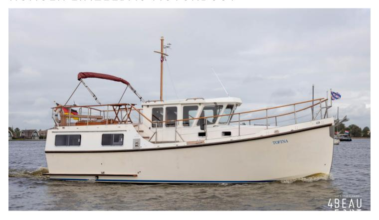
Year built 2006 Length 11.20 meter Width 3.70 meter Draft 1.00 meter Vertical clearance 2.90 meter Reference 4B258
