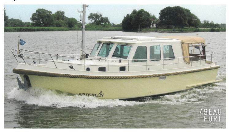
Year built 2003 Length 11.10 meter Width 3.50 meter Draft 0.85 meter Vertical clearance 2.45 meter Material Steel Reference
